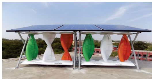
Figure 19 Solar wind hybrid system
