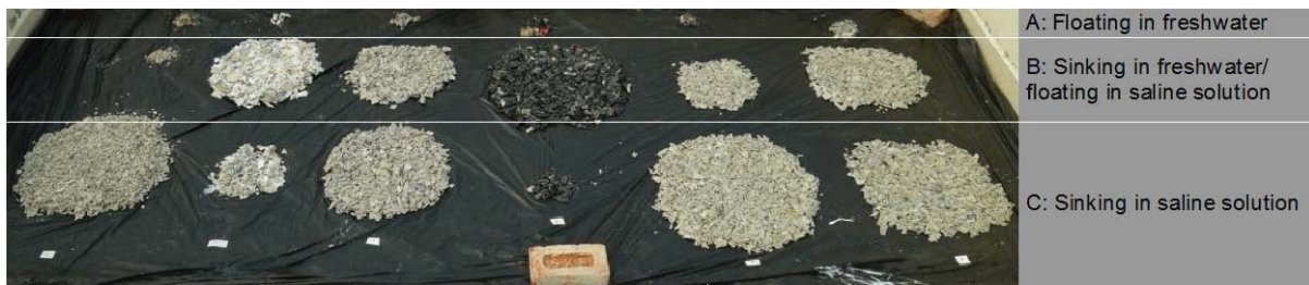
Figure 18: Drying of sub-samples after two-step density separation
