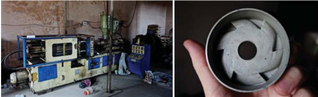
Figure 17: Injection moulding machine (left) and recycled plastic part used in water pumps (right)
