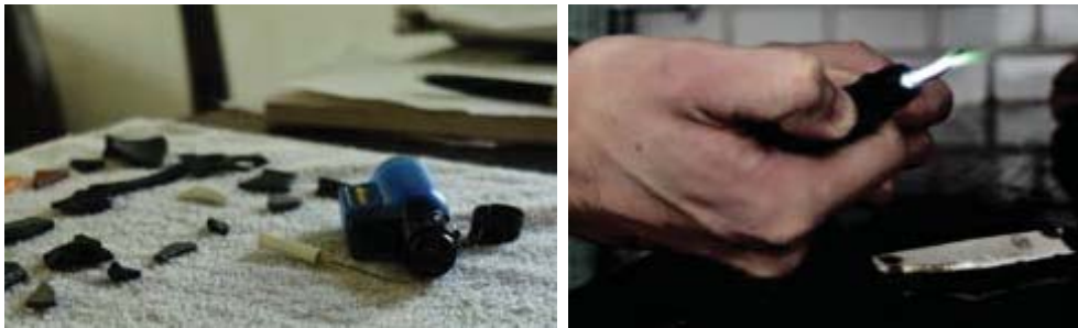
Figure 2: Beilstein test to detect BFR plastics
