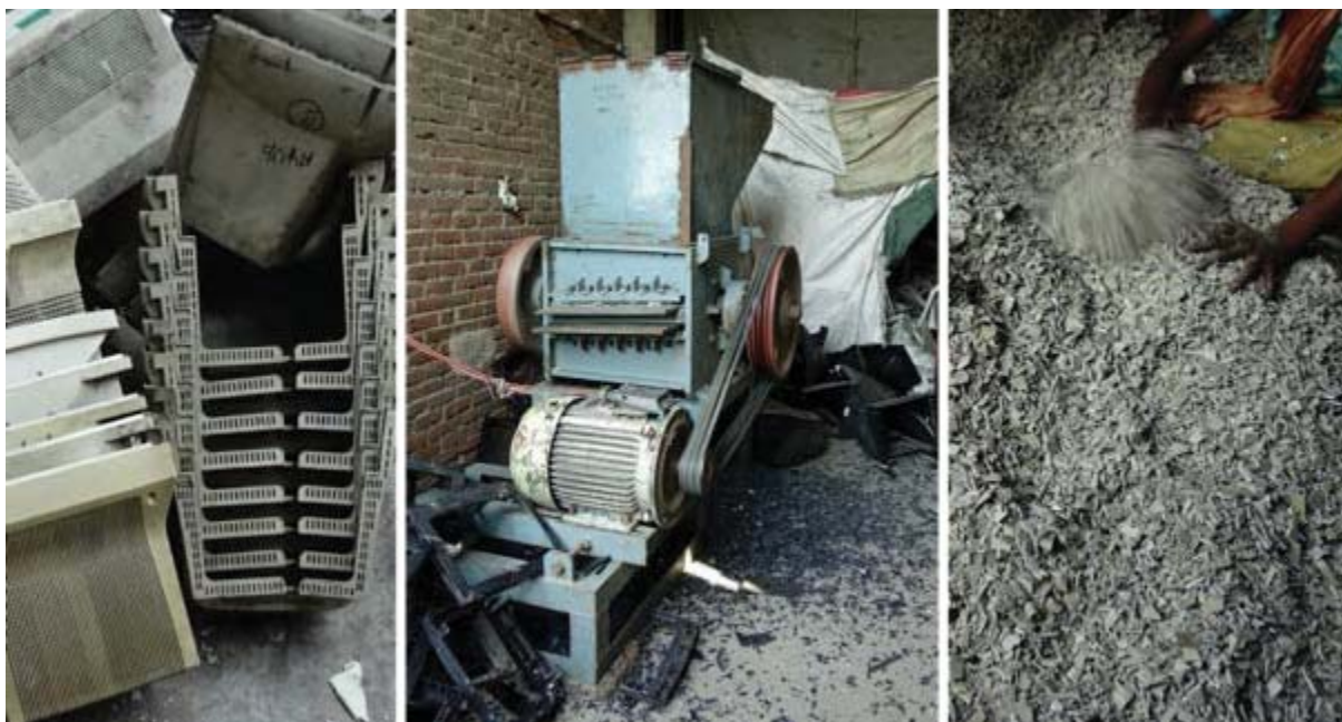
Figure 12: From left to right: Sorted plastic scrap (ABS from CRT monitors); shredder; plastic flakes
