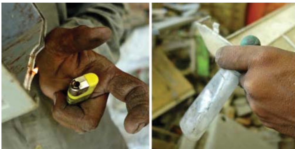
Figure 9: Burn test, to assess flame retardancy (left), and solvent test, to identify plastic type (right)
