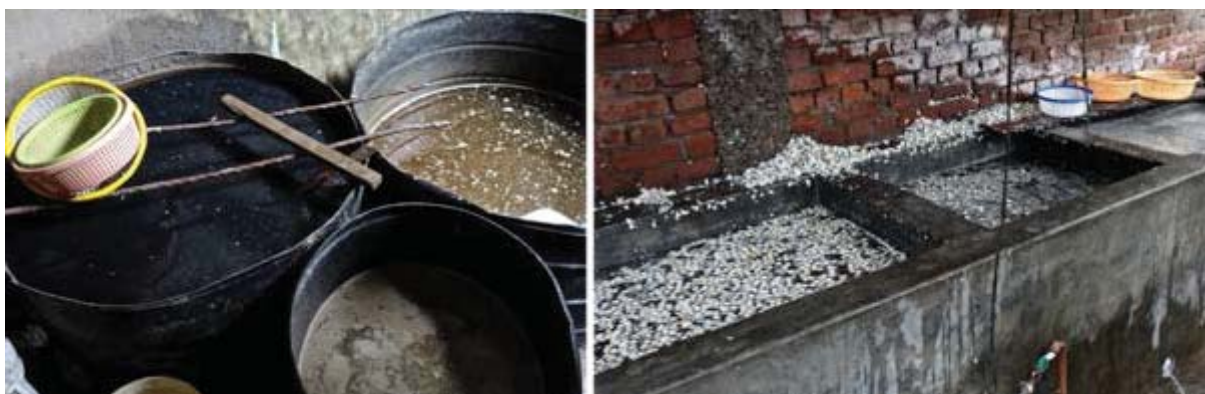
Figure 14: Multi-step density separation using the sink/float method
