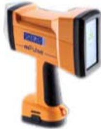
Figure 5: Handheld LIBS (Oxford Instruments, 2015b)
