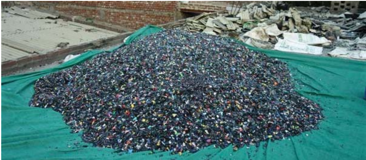
Figure 15: Drying of plastic flakes (here, ABS from household articles and automotive parts)
