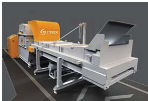
Figure 6: Automated XRT sorting machine (Titech, 2015)
