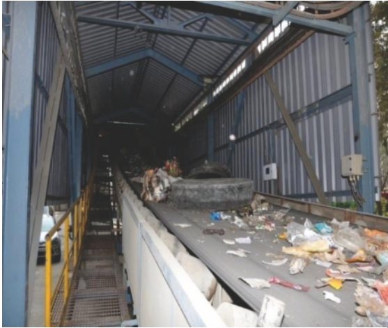
Fig: RDF & waste tyre handling system
