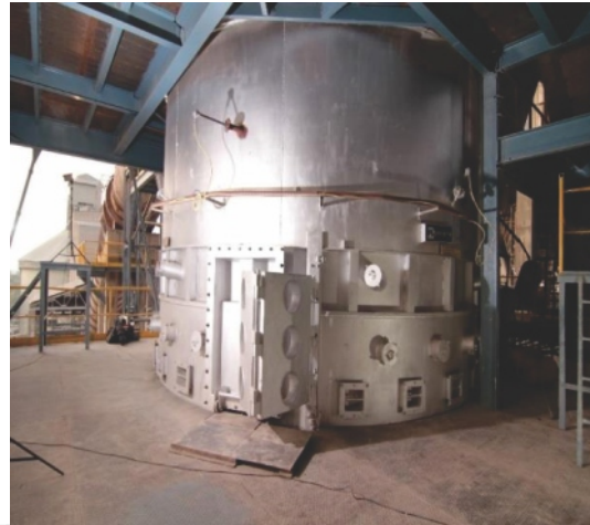
Fig: Hot disc reactor at Vasavadatta Cement.
