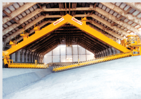
PORTAL SCRAPER RECLAIMER
